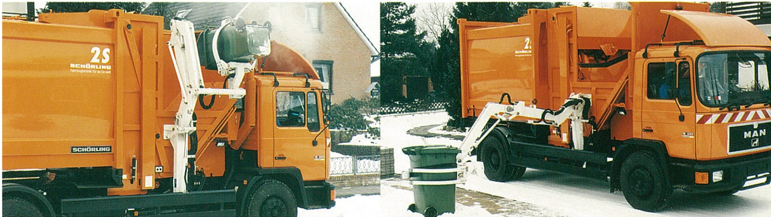
Schorling side-loading vehicle with Manco SL60 arm, working in Hauslingen, Germany.
